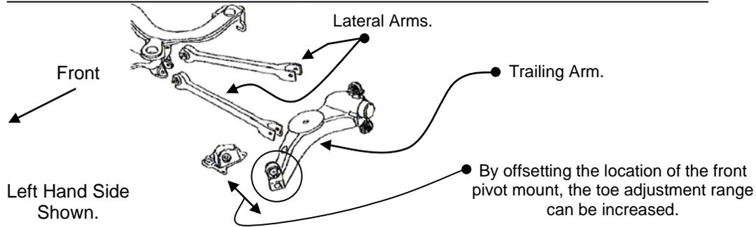
SPF2536K - Rear Trailing Arm Front Bush Kit (Replaces OEM Part No 1J0505171B) Fits All Wheel Drive variations of the VAG A4 Chassis as used on the following models:
