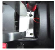
Install the armrest with the two screws provided.
