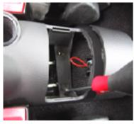
Remove the driveshaft tunnel cover; remove screws.
